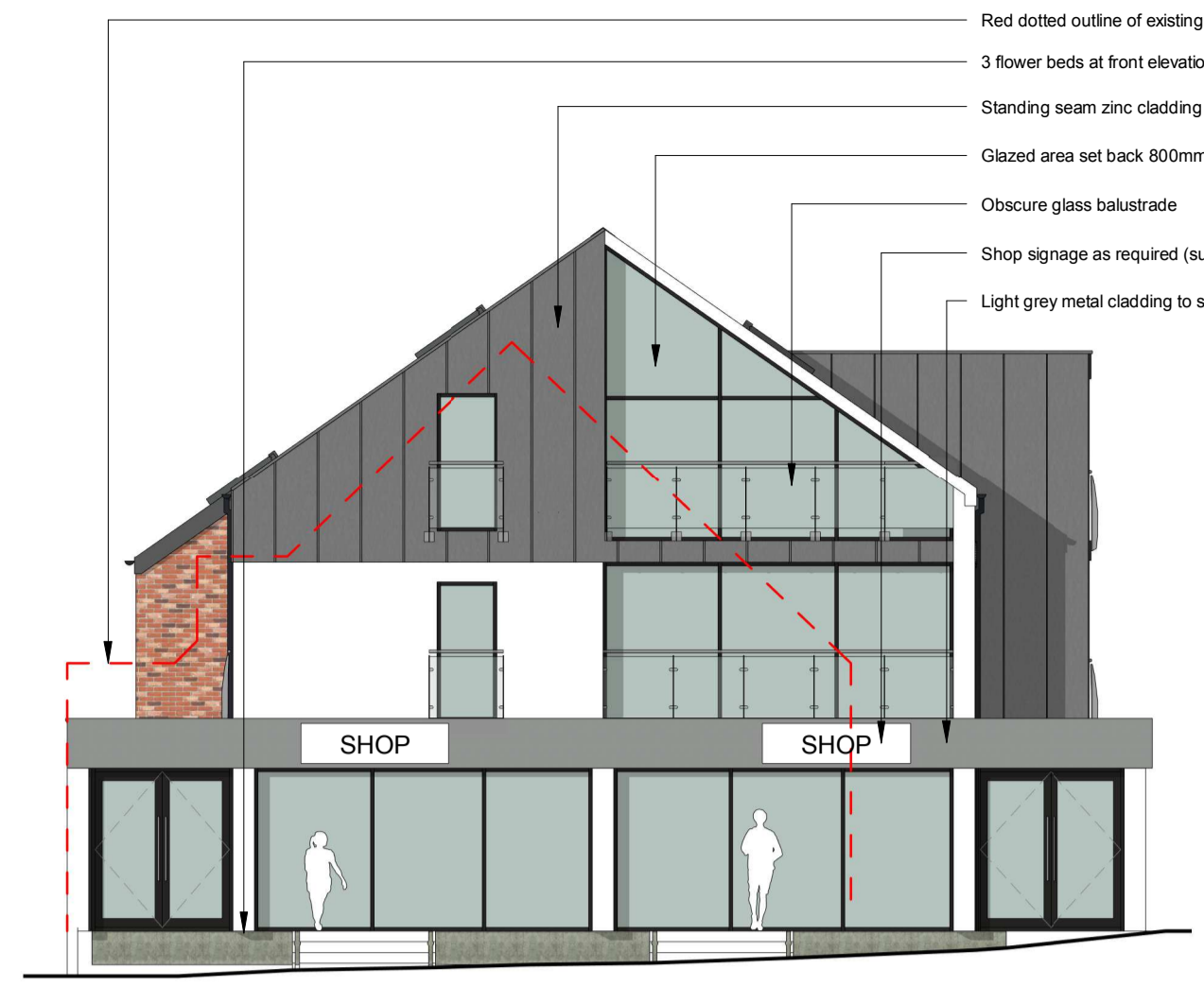
Pantbach Road Elevation 1 : 100
